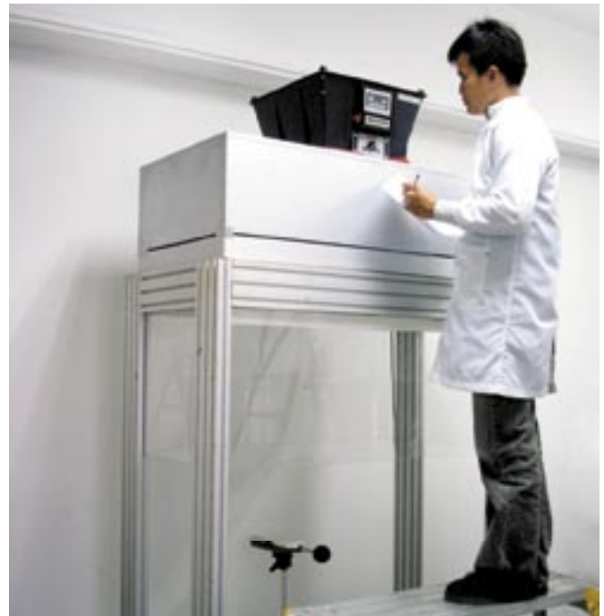
Above: R&D testing at Esco's research laboratory with airflow and noise level test instrumentation
